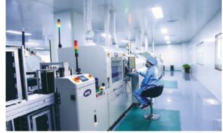
PCB board conformal coating production line
