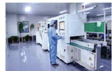
PCB board debugging -FCT and ICT function test production line
