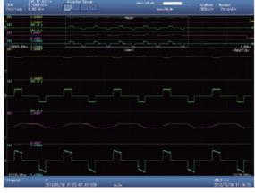
Single charge and discharge test waveform
