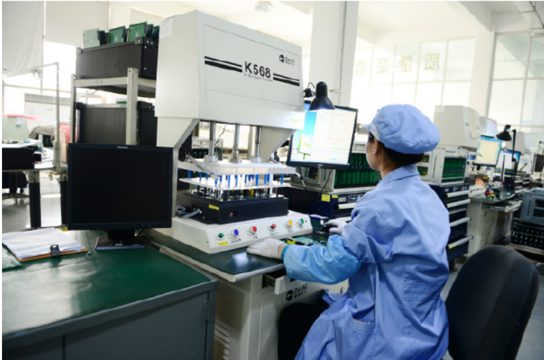
FCT circuit board performance test
