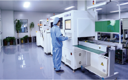
PCB board testing-FCT, ICT functional test line
