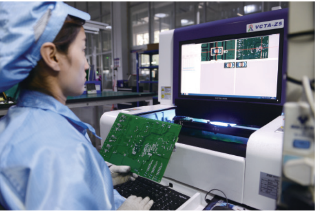
Wave soldering-AOI automatic optical inspection
