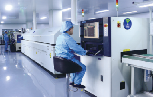
SMT-AOI automatic placement-optical inspection line
